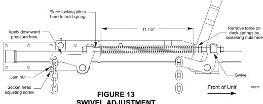
SWIVEL ADJUSTMENT SPRING COMPRESSION ADJUSTMENT
